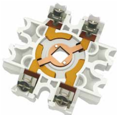
Double bridge Rotor contact Knife type Fixed contacts with self-cleaning effect.
